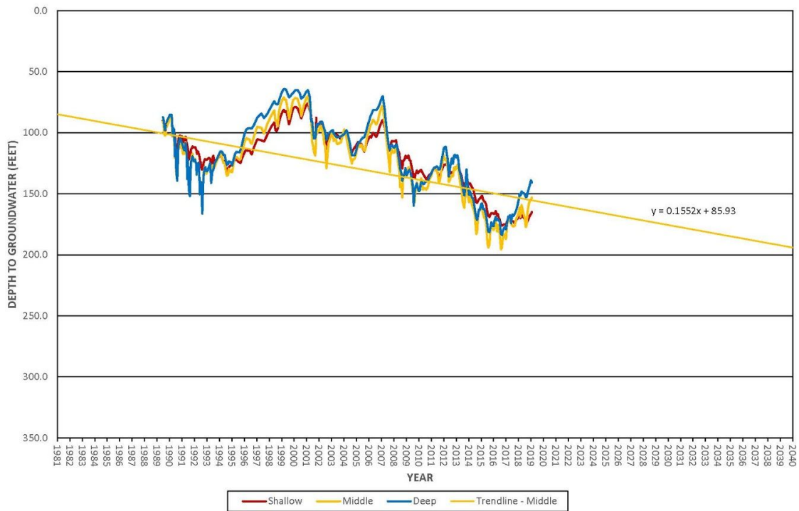
Figure 11. South of River Monitoring Zone Hydrographs
