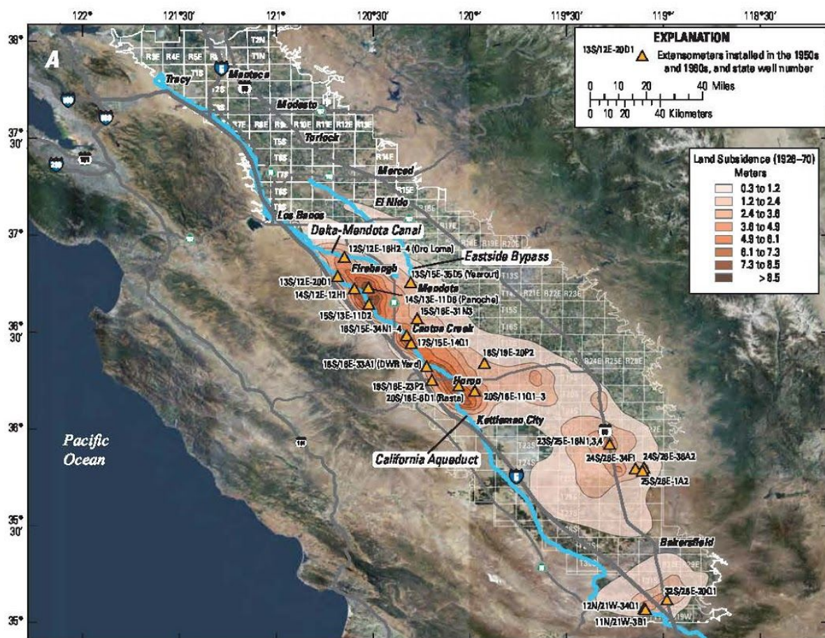
Figure 25 - USGS 1926-1970 Historical Subsidence Areas
