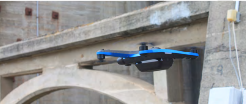
HDR’s California-based drone pilots and data acquisition specialists give IRWD enhanced visibility into hard-to-access work areas, improving progress verification, quality control, and construction documentation throughout the project.
