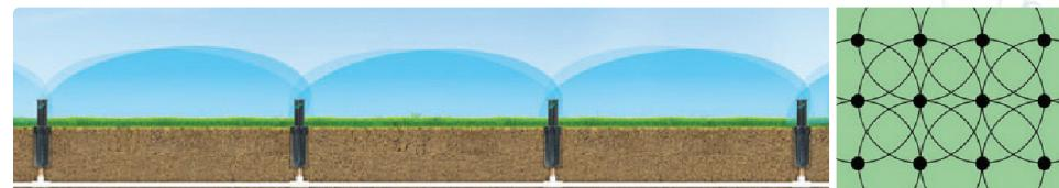
For even coverage, spray heads should be spaced evenly apart the same distance as the range of the spray.
