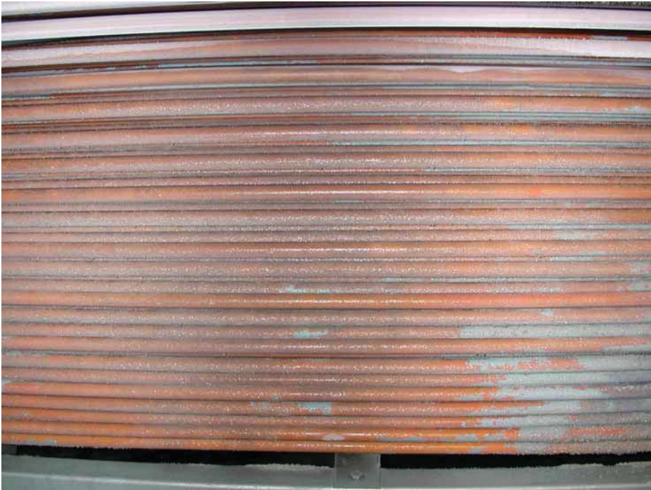
Figure 44: Arcadia tubes after 6 weeks (Nov 26, 2002)
