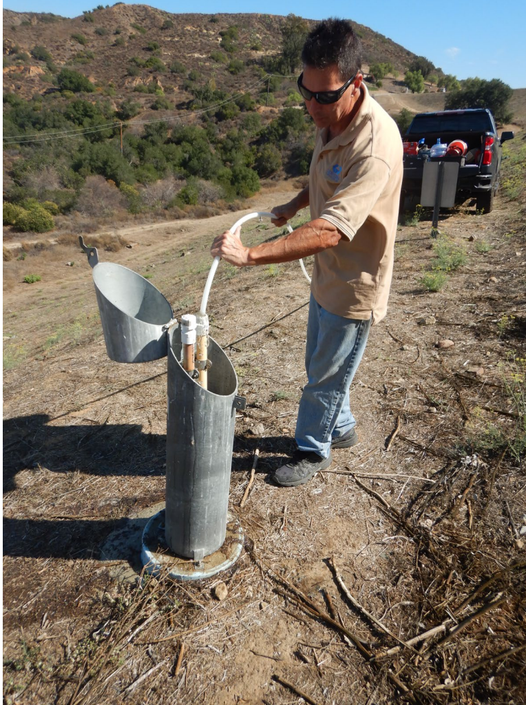
Photograph 5: View of flushing with clean water at Piezometer R-7 Upper.
