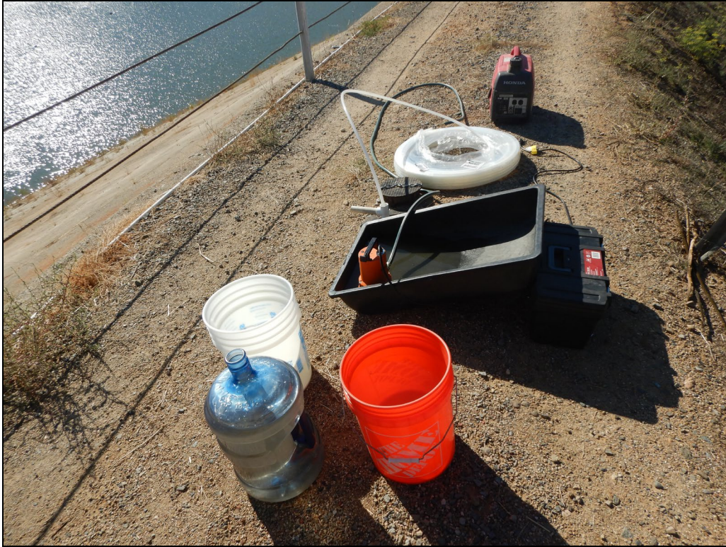
Photograph 2: View of flushing process being performed in Piezometer R-3 Middle at Santiago Creek Dam.
