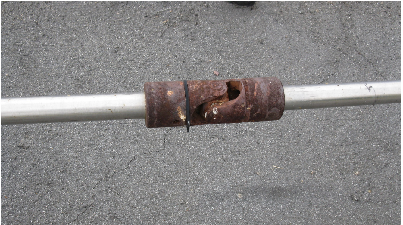
Typical Corroded U-Joints
