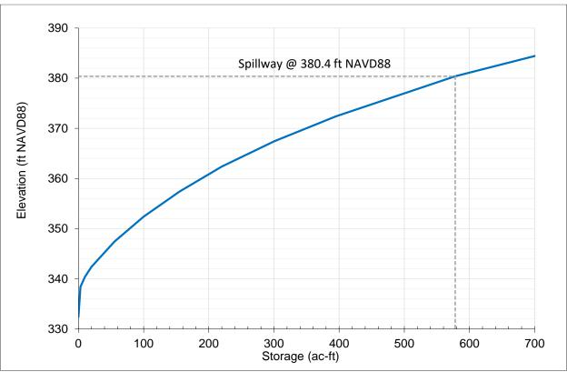
Figure 4-2 Reservoir Storage Capacity Curve
