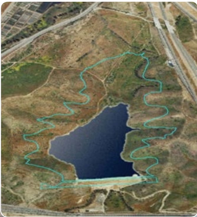
Projected increase in storage capacity of Syphon Reservoir from 500 acre-feet to 5,000 acre-feet.
