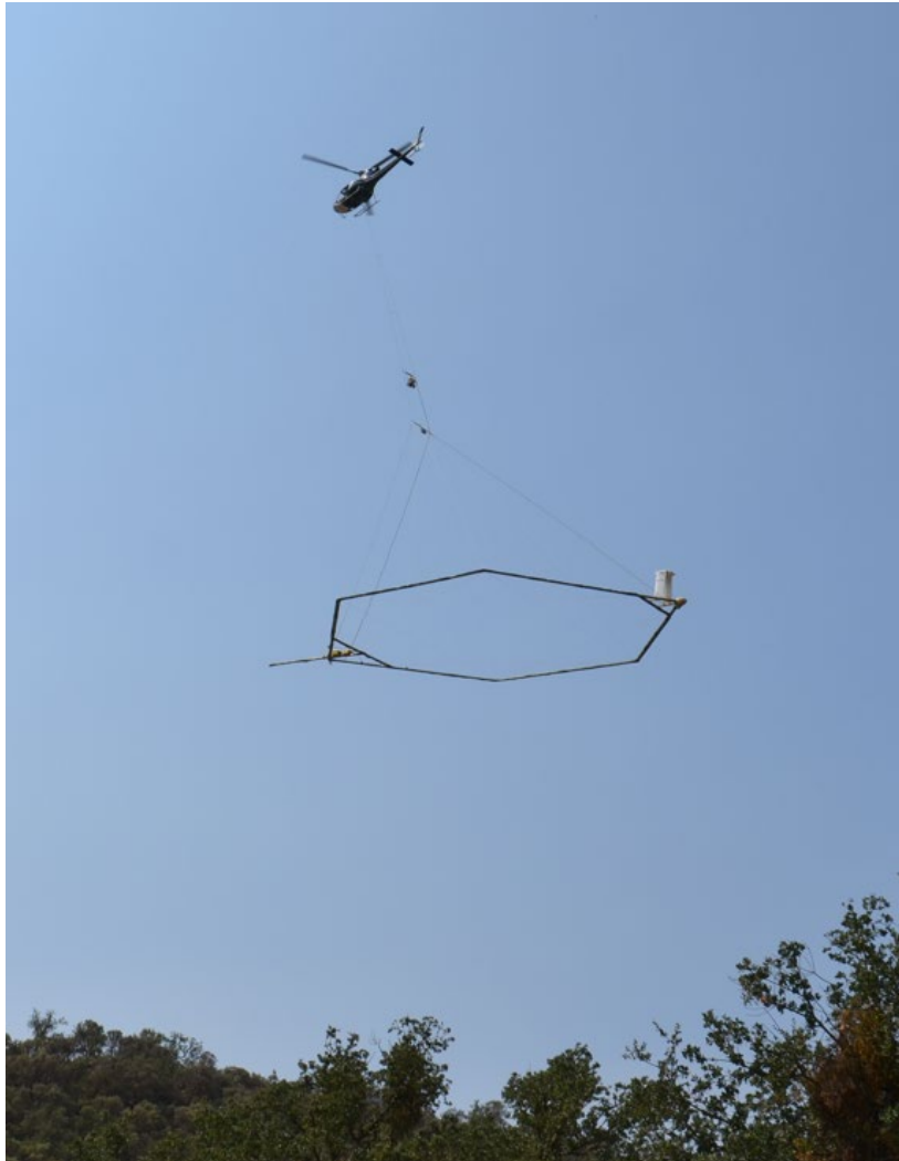
Figure 0-2 Helicopter towing the hexagonal SkyTEM system while collecting AEM data during the survey.
