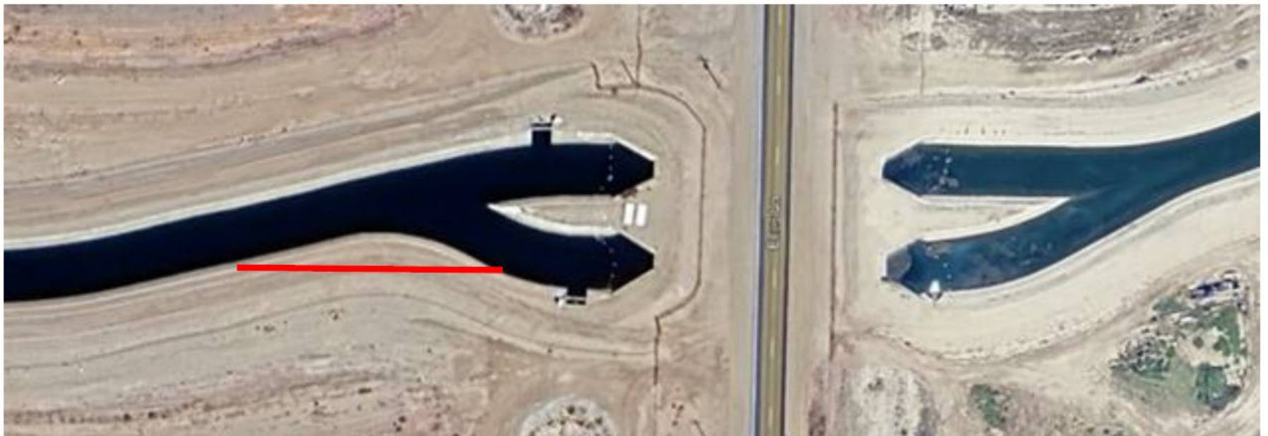
Figure 4. Enos siphon widening recommendation
