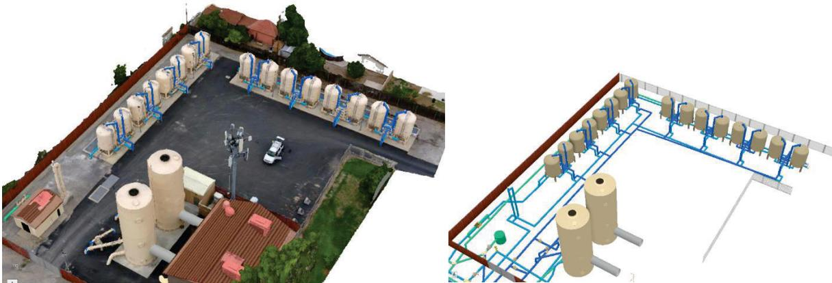
Figure 9 – Left side - Sample Drone Model overlaid with UN Data, Right side – UN data in 3D View , refined per Drone model.
