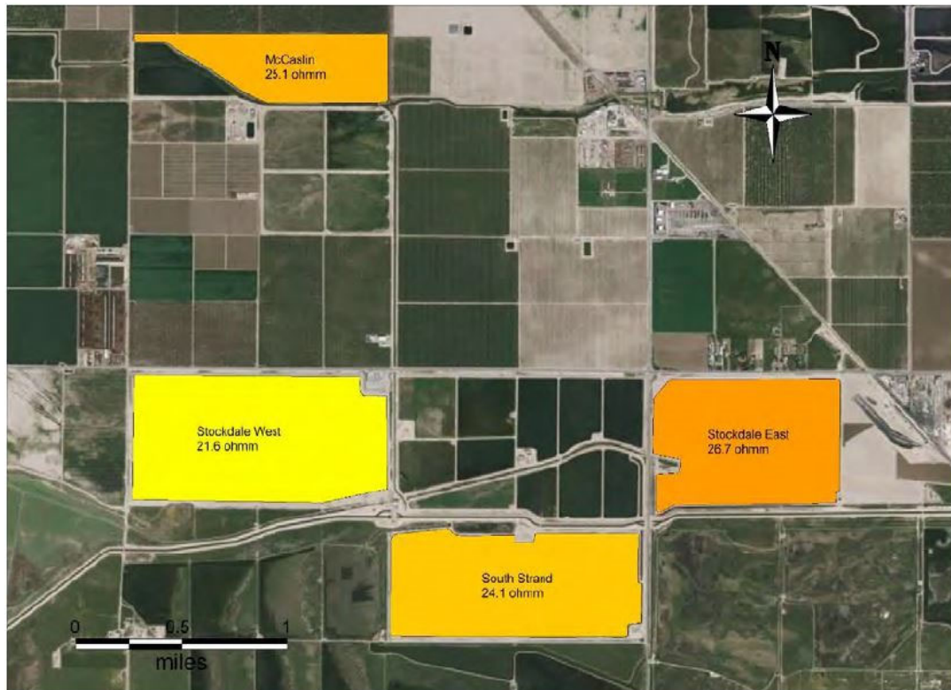
Figure 3: Average Resistivity for McCaslin Property (Portion of Phase I)
