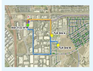
The left image shows two potential pipe routes to convey raw water from the Tustin Legacy Well Area 1 and 2 to the Well 21/22 Treatment Plant. It also shows the location where the distribution system will see increase flows (X) as a result of the additional well supply.
