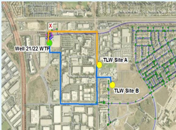
The left image shows two potential pipe routes to convey raw water from the Tustin Legacy Well Area 1 and 2 to the Well 21/22 Treatment Plant. It also shows the location where the distribution system will see increase flows (X) as a result of the additional well supply.
