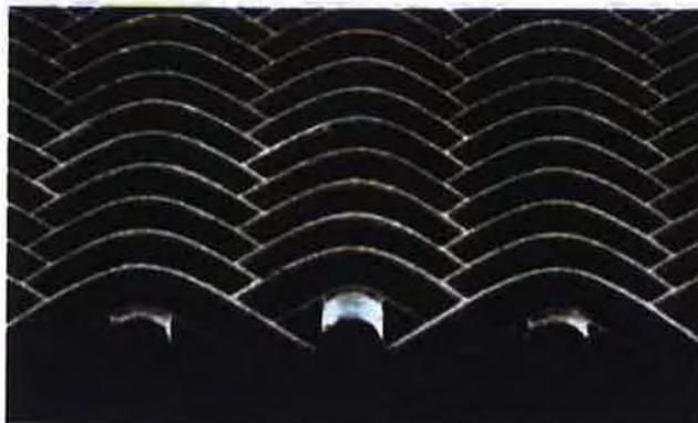
*10-Micron Weave Wire Strainers would perform well as a second stage screen.*
