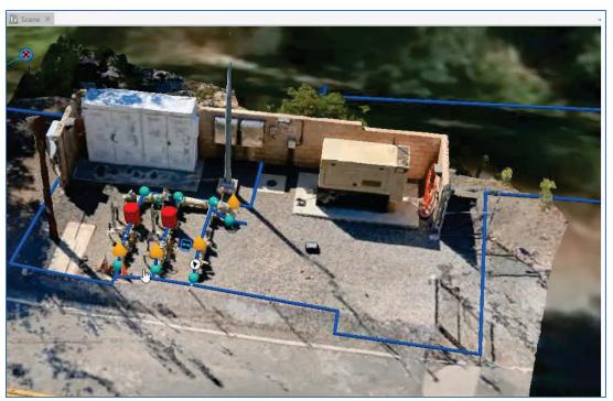
Figure 12 - Pump Station Reality Capture Combined with Utility Network
