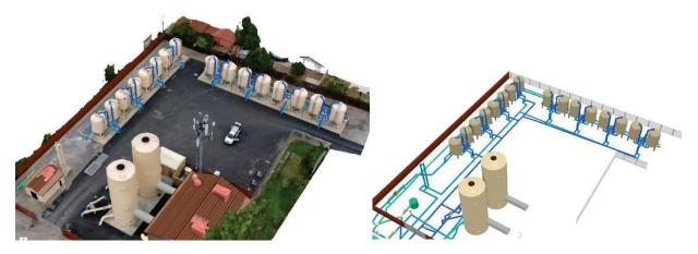
Figure 9 – Left side - Sample Drone Model overlaid with UN Data, Right side – UN data in 3D View, refined per Drone model.
