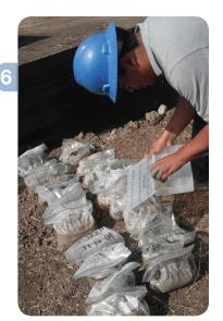
Drill cuttings (soil samples) used to classify the types of soil found at various depths of the well.
