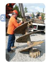
In preparation for borehole drilling, the bucket auger drill is attached to a drill rig.
