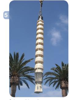
Submersible well pump before installation.
