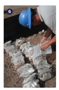
Drill cuttings (soil samples) used to classify the types of soil found at various depths of the well.
