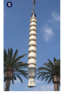
Submersible well pump before installation.
